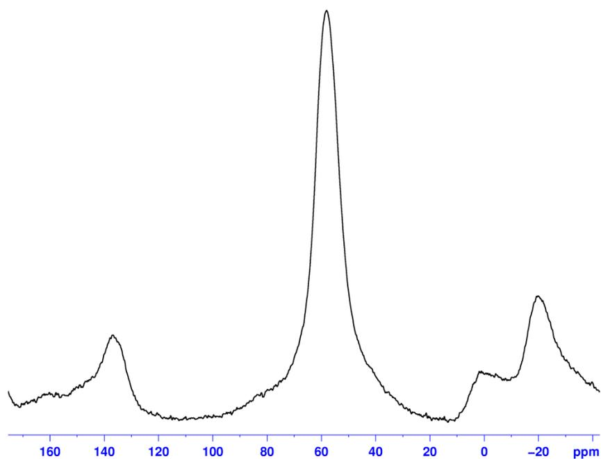
$^{27}\text{Al}$  spectrum of geopolymer, spinning rate 10 kHz.  $^{27}\text{Al}$  MAS NMR spectroscopy is able to recognize coordination number of Al in silico-aluminates. Four coordinated aluminium resonates at approximately 50 ppm while six coordinate aluminium resonates at about 0 ppm.
