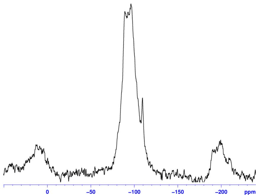
$^{29}\text{Si}$  spectrum of geopolymer, spinning rate 10 kHz. Spectrum can be used to determine Si connectivity.
